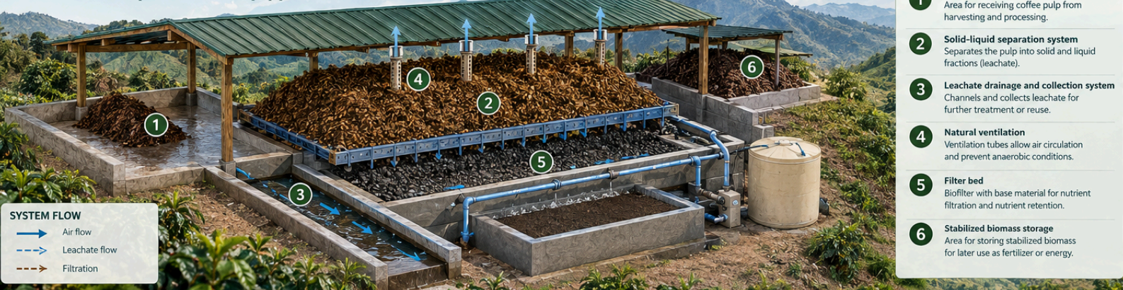
Figure 7.2 Passive infrastructure implemented for coffee pulp preservation.
